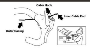
Route the cable through the housing and into position and secure the housing to the bar.
