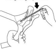
3. Once positioned, tighten the 5mm Allen bolt to 6-8 Nm.
