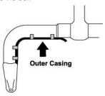
Finally, route the cable through the brake and adjust to the brake manufacturers specifications, and secure the brake.
