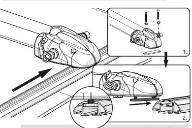
Take out the rubber strap and slide the T-blots into the roof bar slot, then cutting the rubber strap with appropriate length and insert it back.
