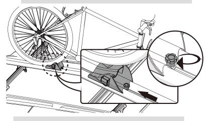
Use the ratchet strap to secure the wheel with cushion pad.
