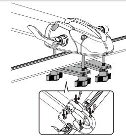
Place the front fork onto the quick release skewer. Fix one side by turning the knob.
