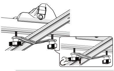
Use the knobs to fix the cross bar between tray and rear bracket.
