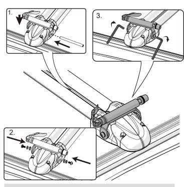
Place the front fork onto the quick release skewer. Fix one side by turning the knob.
