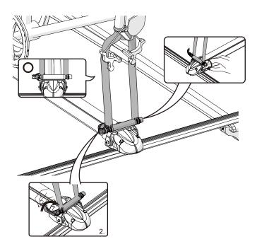
Push the wheel tray for proper fit of bike wheel then tighten the knob to fix the position.
