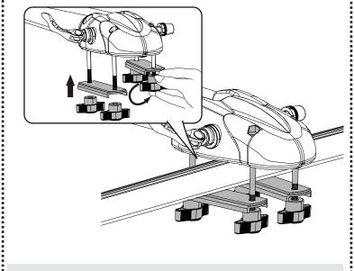
Use the knobs to fix the cross bar between front housing and front bracket.
